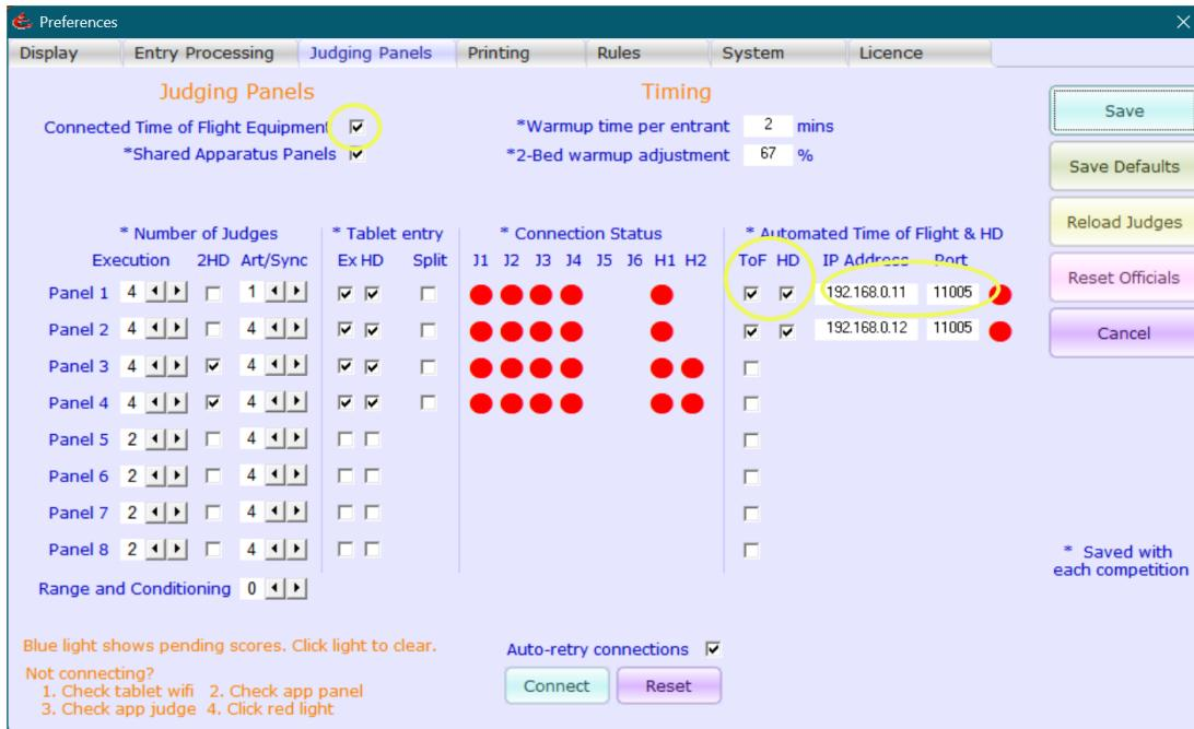
Then pick the ToF and HD boxes for each of panels that are using the QIRA system and fill in the IP Address and Port number to use. (To find the IP Address of the QIRA computer, just start a command shell and type `ipconfig`. The IPv4 value should be of the form 192.168.x.y. Alternatively, the QIRA network config screen shows its IP address.
