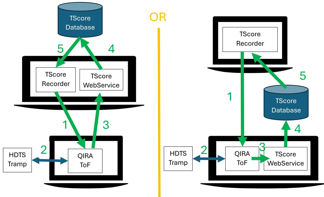
To communicate, each of the components has to know which computer the other component is running on (Its IP Address) and the number of the 'port' that the other computer is monitoring for data.
